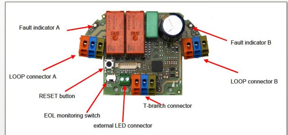
The FIM is equipped with a power capacitor that is charged by the LDB and has enough capacity to run at least two measurement cycles without the need for re-charging. The LED indicator(s) on the FIM are flashing with intervals to indicate quiescent or fault condition. The FIM has a RESET button and EOL-enable switch. Please refer to the User and Installation manual V01R01 for detailed information.
