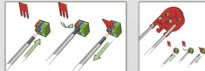
The FIM is equipped with WAGO push-terminals that accept up to 2,5 mm<sup>2</sup> core installation cable. A special tool is provided to quickly remove all three wires in one run. (Release-tool is included)
